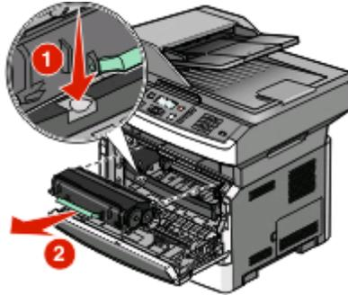
Press the button on the base of the photoconductor kit. Pull the toner cartridge up and out using the handle.
