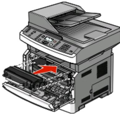
Insert the toner cartridge into the photoconductor kit by aligning the rollers on the toner cartridge with the tracks. Push the toner cartridge until it *clicks* into place.
