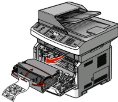
Remove the photoconductor kit and toner cartridge from the printer.
