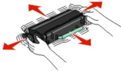
Firmly shake the cartridge side to side and front to back several times to distribute toner.
