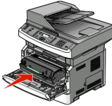
Reinsert the photoconductor kit and toner cartridge into the printer.
