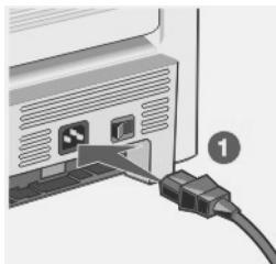
Connect the power cord to the printer and then to a properly grounded outlet that is near the printer and easily accessible. Turn the printer on.
