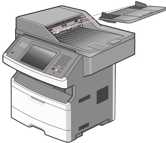
Attach the ADF tray to the printer.
