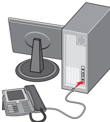
6 Conecte um cabo adicional de telefone da porta do modem do computador até a
