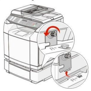
**6** Loosen the left thumbscrew, and remove the left bracket.
