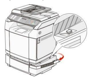
Remove the left side cover by starting at the back of the printer and gently pulling each of the four slots off of its matching tab as you work your way to the front of the printer.
