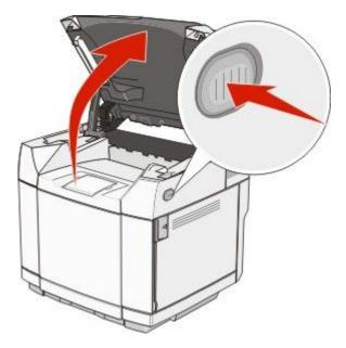
**5** Push the latches toward each other to release the photodeveloper cartridge.
