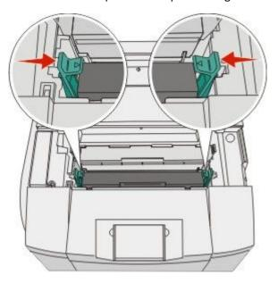
Grasp the handle, and pull the photodeveloper cartridge straight up and out.
