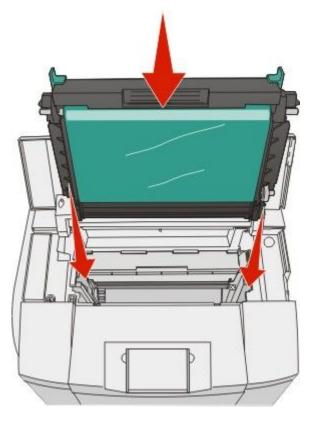
11 Push the latches away from each other to lock the photodeveloper cartridge into place.
