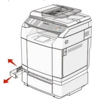
Loosen the right thumbscrew, and remove the right bracket.
