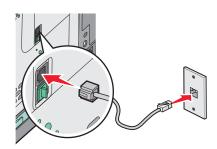
**3** Remove the protective plug from the bottom EXT port  $\widehat{\ }$  of the printer.
