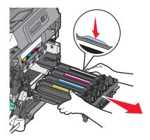
Remove the used developer unit.
