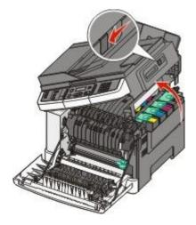
**4** Remove the toner cartridge by lifting the handle, and then gently pulling away from the imaging kit.
