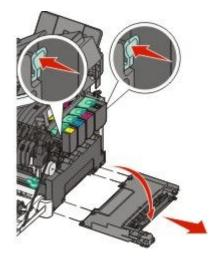
**5** Press the green levers on each side of the waste toner bottle, and then remove it.
