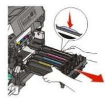
8 Remove the used developer unit.
