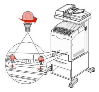
**5** Lift the printer off the drawer, and set the printer aside.
