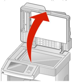
Open the bottom ADF door, and then remove any jammed pages.
