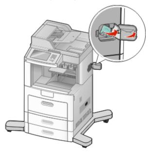
Pull the latch of the staple cartridge holder down, and then pull the holder out of the printer.
