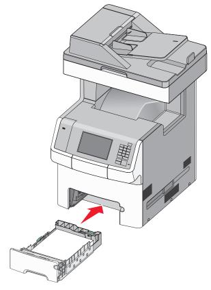
7 From the printer control panel, verify the paper size and paper type setting for the tray based on the paper you loaded.
