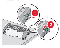
$\boldsymbol{f}$  Press the green arrow tab to the left, and then lift the top paper guide.
