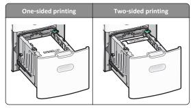
• Make sure paper does not exceed the maximum paper fill indicator located on the side of the tray.
