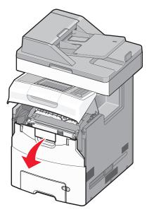
**Warning—Potential Damage:** To avoid overexposing the photoconductor units, do not leave the front door open for more than 10 minutes.
