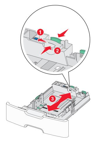
**3** Squeeze and slide the width guide to the correct position for the paper size you are loading.
