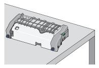
e Pull and then rotate the green rectangular knob clockwise to unlock the top paper guide.
