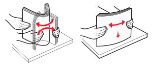
**5** Load the paper stack toward the back of the tray with the recommended printable side faceup.
