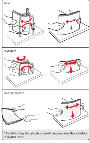
**4** Load the paper or specialty media. Slide the stack into the multipurpose feeder until it comes to a stop.
