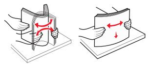
**6** Load the paper stack with the recommended printable side faceup.
