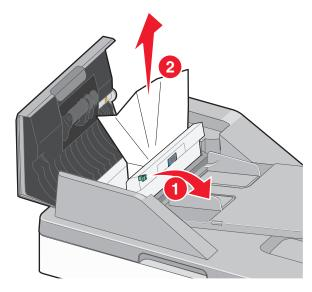
**5** Open the scanner cover, firmly grasp the jammed paper on each side, and then gently pull it out.
