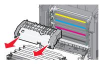
**d** Place the fuser on a flat surface with the blue thumb screws facing you.
