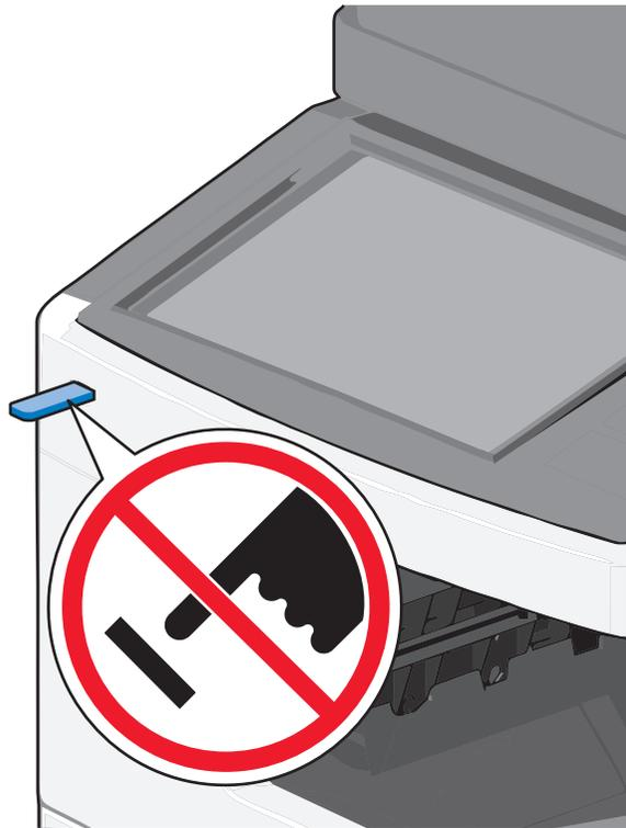
**Warning—Potential Damage:** Do not touch the USB cable, any network adapter, any connector, the memory device, or the printer in the areas shown while actively printing, reading, or writing from the memory device. A loss of data can occur.
