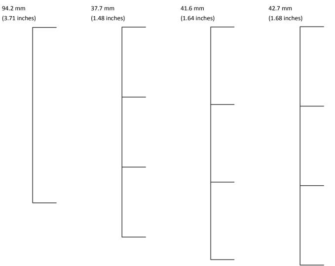
Change the transfer module if one of these defects appears on the printed page. Change the fuser if one of these repeating defects
