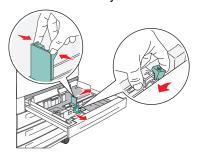
**3** Squeeze the front guide tab, and slide the guide to the correct position for the media size you are loading.
