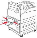
7 Set the Paper Size and Paper Type for the multipurpose feeder (MP Feeder Size and MP Feeder Type) to the correct value for the print media you loaded.
