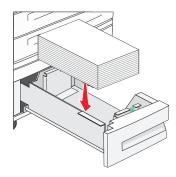
**Note:** Make sure the print media is below the max fill line on the rear guide. Overloading may cause jams.
