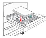
**6** Squeeze the side guide tab, and slide the guide until it lightly rests against the edge of the media.
