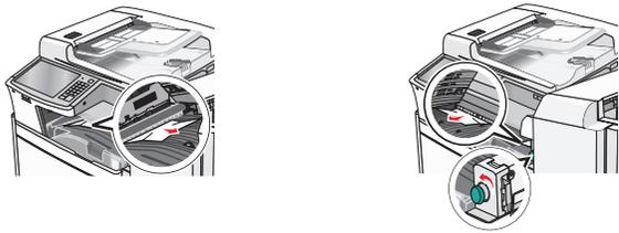
**Note:** If the paper jam on the right is difficult to remove, then rotate the knob counterclockwise.
