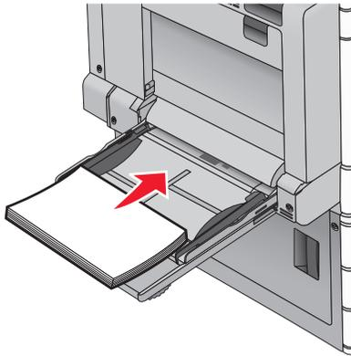
**Warning—Potential Damage:** Pulling the paper out, without pushing the paper pick tab first, may cause jams or the paper pick tab to break.
