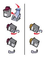
**Warning:** Do *not* touch or remove the gold contact areas on the back and bottom of the cartridges.
