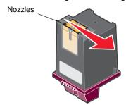
4 Hold a clean, damp section of cloth against the contacts for about three seconds. Gently blot and wipe dry in one direction.
