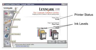
The Lexmark Solution Center consists of six tabs: Printer Status, How To, Troubleshooting, Maintenance, Contact Information, and Advanced.
