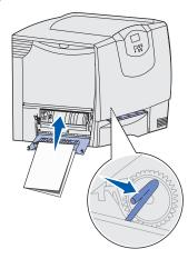
**3** Close the left access door and the front access door. If the jam persists, continue with step Turn the printer off. Open the front cover..
