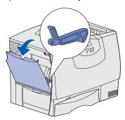
**2** Press the pick assembly release lever, and remove all media and jams.
