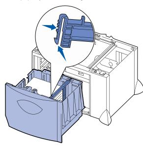
3 Squeeze the two front guide levers and slide the guide to the correct position for the size paper you are loading.
