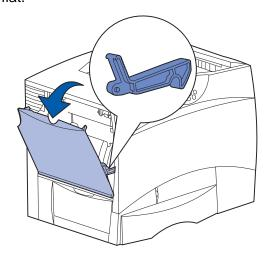
2 Remove any jams and return the feeder to its working position.
