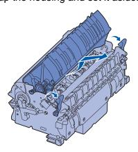
6 Lift up the fuser roller cover and remove the jam.
