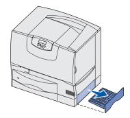
2 Remove any jams, and then reinstall the tray.
