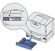
**2** Reinstall the duplex mechanism in the printer.
