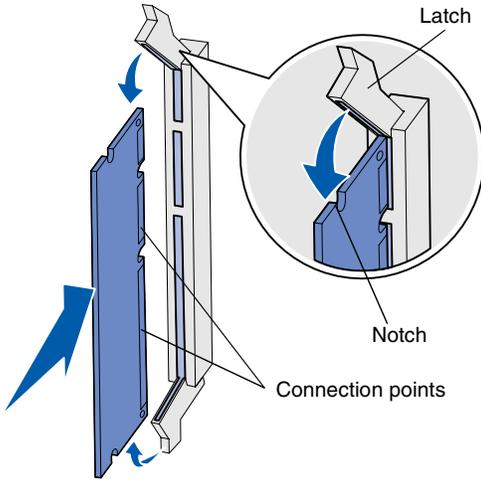
Follow the instructions in this section to install a printer memory card. Memory cards must have 168-pin connectors.
