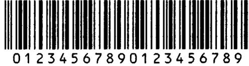
Interleaved 2of5 is used to express all-numeric messages. Two bytes of data are encoded to form one barcode character. If the check digit generation flag is on ( $b_0 = 1$ ), the printer will add a '0' to the data string automatically.
