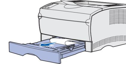
If you see any print media above the metal stop, completely remove the tray. Press down on the print media to lock the metal plate below it into place. Reposition the print media under the metal stop.
