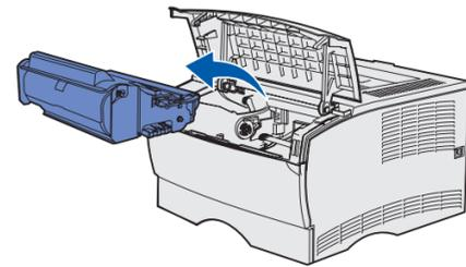
**Warning!** Do not touch the photoconductor drum on the bottom of the print cartridge.
