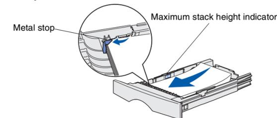
**Note:** Do not exceed the maximum stack height. Overfilling the tray may cause a jam.
