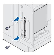
6 Align the connection points on the card with the connector on the system board and push the card firmly into the system board connector.
