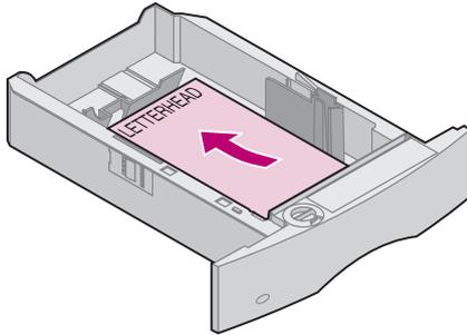
For *duplex* printing on letterhead paper, place the printed design side *face up* with the top of the page nearest the length guide.
