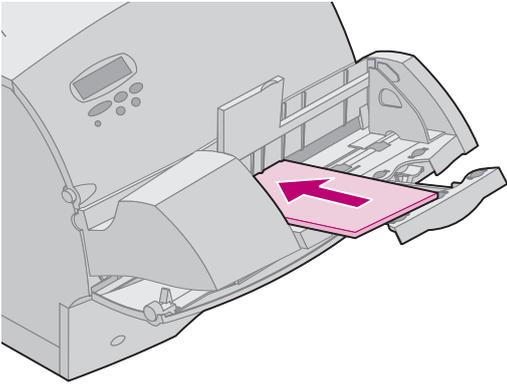
**7** Load the stack of envelopes with the address side up and flap side down. The flap side edge of the envelope should be facing the left side of the envelope feeder. Make sure the envelopes at the bottom of the stack slide into the envelope feeder slightly more than the ones at the top of the stack.
