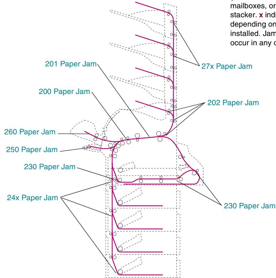
**Note:** **27x Paper Jam** may occur in any output option: output expanders (shown in illustration), 5-bin mailboxes, or high-capacity output stacker. **x** indicates the output option depending on how many you installed. Jam areas shown may occur in any output option.
