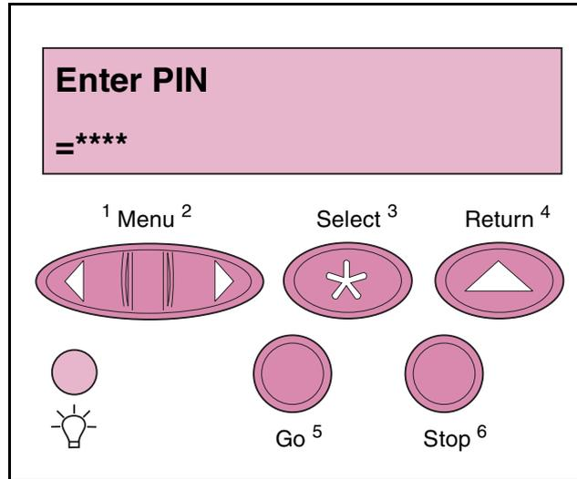
If you enter an invalid PIN, the message **No Jobs Found. Retry?** displays. Press **Go** to reenter the PIN, or press **Stop** to exit the Confidential Job menu.
