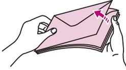
6 Straighten the edges on a level surface. Press down the corners to flatten them. Fan the envelopes. This prevents the edges of the envelopes from sticking together and helps them feed properly.
