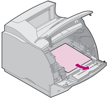
**NOTE:** If there is resistance to the paper, and it does not move immediately when you pull, stop pulling. You need to access the paper from the rear door. See [“202 Paper Jam Open Rear Door”](#) on [page 74](#) for more information.
