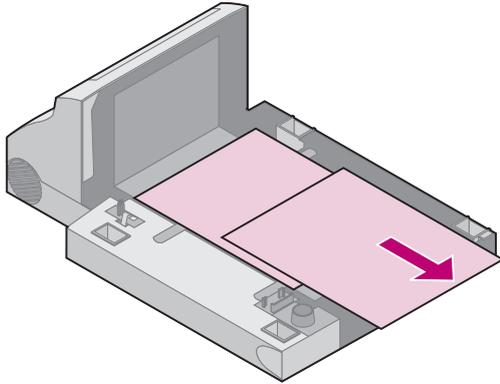
Up to two sheets of paper are lying behind the duplex front access cover inside the duplex unit.
