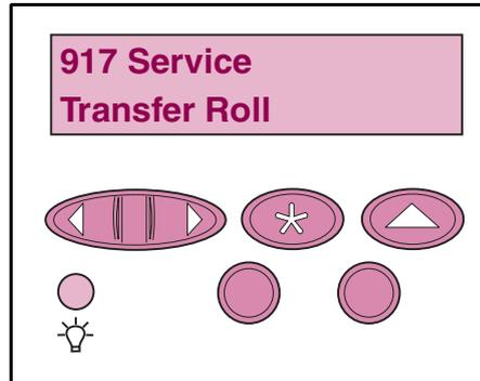
A service message indicates a printer failure that may require a service call.
