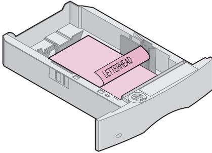
For *simplex* (single-sided) printing on letterhead paper, place the printed design side *face down* with the top edge of the page nearest the knob for the paper size indicator.
