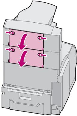
Paper jams as it exits to an output option tray and a short portion of the paper is visible.
