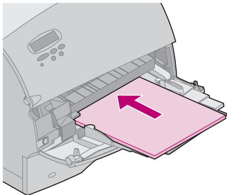
**6** Slide the print material into the multipurpose feeder as far as it will go. Do not force it. Forcing causes buckling of the print material.
