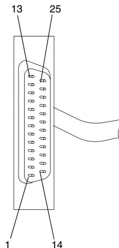
The following illustration shows the pin assignments for the 9-pin to 25-pin IBM EIA RS-232C serial cables.
