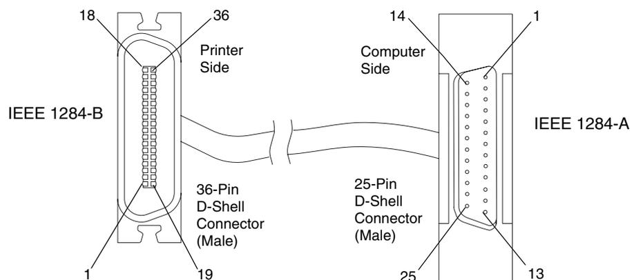
The following illustration shows the pin assignments for connecting the 25-pin connector to the 36-pin connector. The symbol \* indicates an active low signal.
