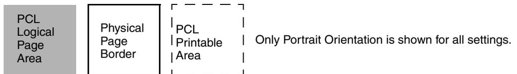
The *Normal* setting, which is the factory default, means the printable area includes the entire page except the narrow border around the edge of the page. This is the nonprintable area. The printer measures margin settings relative to the logical page.
