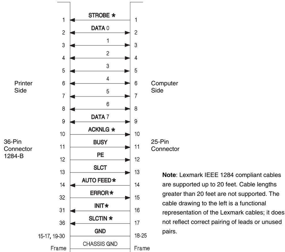
The parallel interface consists of an 8-bit parallel data bus with the following characteristics:
