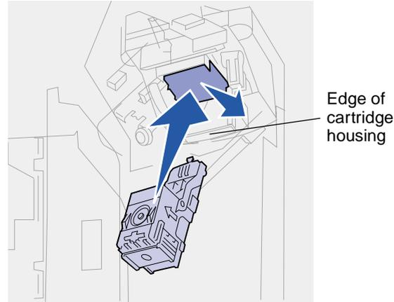
**Note:** When the staple cartridge holder is correctly placed, the lever on the stapler moves to its original position.
