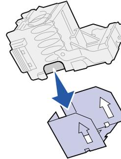
5 Insert the new staple cartridge into the staple cartridge holder.
