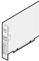
Install a MarkNet N2501e or N2401e internal print server if you received either of these cards as part of a multifunction printer upgrade.
