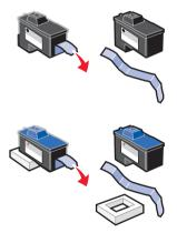
Warning: Do NOT touch the gold contact area on the cartridges.
