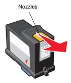
4 Hold a clean, damp section of cloth against the contacts for about three seconds. Gently blot and wipe dry in one direction.
