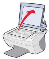
2 Place the item you want to copy face down on the scanner glass. Make sure the upper left corner of the front of the item aligns with the arrow.
