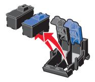
**5** If you are installing new cartridges, remove the foam, stickers, and transparent tape from the bottom of the cartridges.
