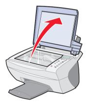
**3** Place the item you want to scan face down on the scanner glass. Make sure the upper left corner of the front of the item aligns with the arrow at the bottom right of the scanner.
