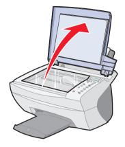
3 Place the item you want to scan face down on the scanner glass. Make sure the upper left corner of the front of the item aligns with the arrow at the bottom right of the scanner.
