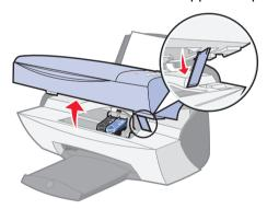
The print cartridge carrier moves and stops at the loading position unless the All-In-One is busy.
