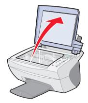
**3** Place the item you want to copy face down on the scanner glass. Make sure the upper left corner of the front of the item aligns with the arrow at the bottom right of the scanner.
