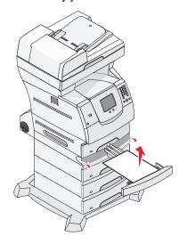
Pull the print media either up or down. If it does not pull easily one way, try the other way
