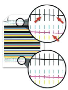
Compare the diagonal lines above the printed bars to the diagonal lines below the printed bars. Look for a break in the diagonal lines above the printed bars. Broken lines indicate clogged nozzles. Look for continuity in the diagonal lines below the printed bars. Unbroken lines indicate clean nozzles.
