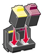
**c** Push back firmly on the cartridge until it **snaps** securely into place.
